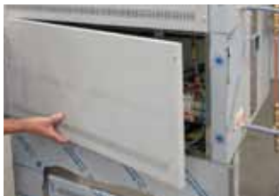
Fig. 4.1 Loosen the screws on the right panel.
