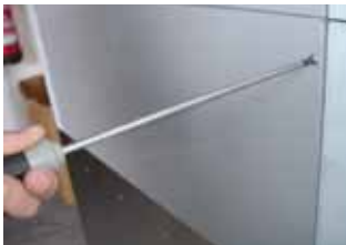
Fig. 2.1 Loosen the screws on the left side panel.
