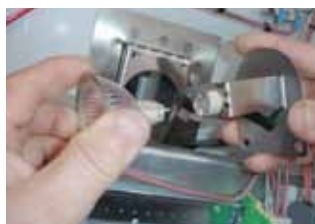
Fig. 4.4 Substitute light bulb.
