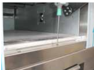
Fig. 5.1 Loosen lower frame screws.
